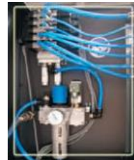
FESTO central air for easy maintenance
