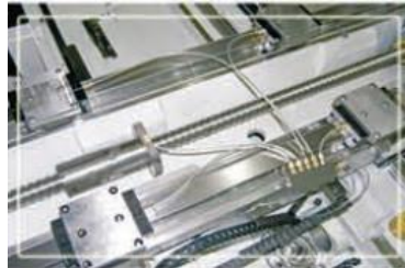
Central lubrication of roller guide and precision ball screws
