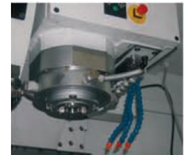
water curtain around spindle
